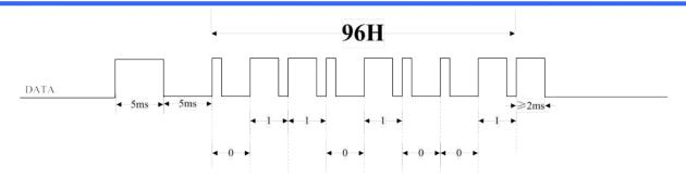
Suppose we want the chip to play the voice content of address 01/02/03/04 in turn. That is to play with the code command, F3+01+F3+02+F3+03+F3+04. The corresponding timing can be as shown in the figure below:
