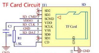
When the chip in the module has a built-in FLASH, TF card can be connected.
