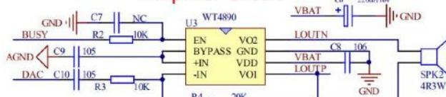
When the chip's own PWM output with 8R 0.5W speaker is selected, no external power amplifier circuit is needed.
