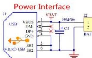
Power supply (3.7V lithium battery and 5V adapter are optional, and charging circuit needs to be added when using lithium battery for power supply)
