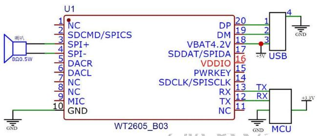
Note: the IO port of WT2605B03-V2.02 is 3.3V level
