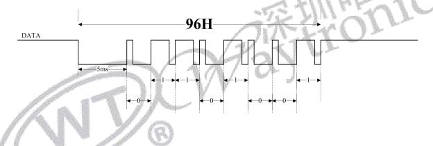
Suppose we want the chip to play the voice content of 01/02/03/04 address in turn. That is, concatenated code instruction playing, F3+01+F3+02+F3+03+F3+04. The corresponding time sequence can be shown in the following figure:
