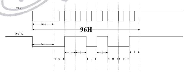
Suppose we want the chip to play the voice content of 01/02/03/04 address in turn. That is, concatenated code instruction playing, F3+01+F3+02+F3+03+F3+04. The corresponding time sequence can be shown in the following figure:
